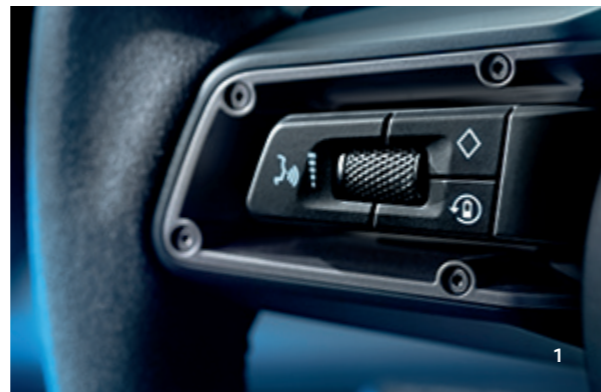
1 Recuperation button on the Steering Wheel for selecting recuperation stages
