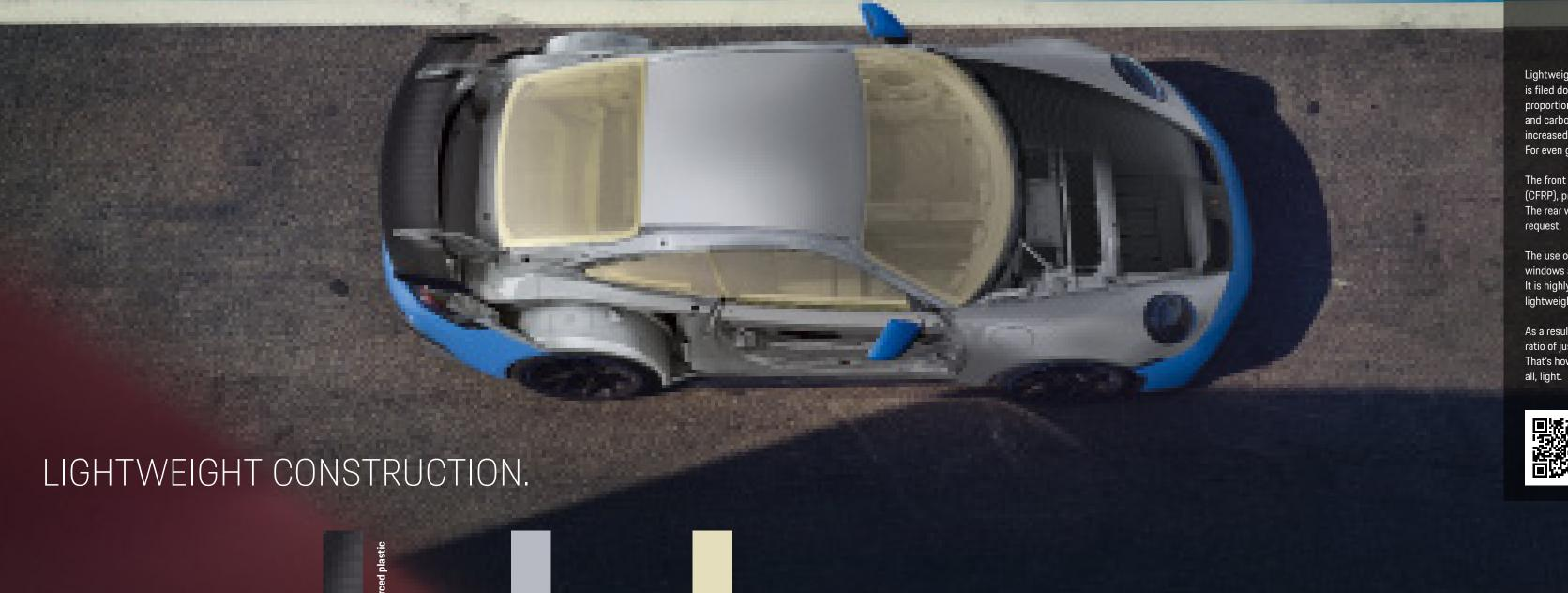
Lightweight construction always goes into detail: every gram is filed down so as to fight for every weight saving. The proportion of lightweight components made of aluminium and carbon-fibre reinforced plastic (CFRP) has been increased once again, while maintaining the same stability. For even greater agility, typical of motorsport.
