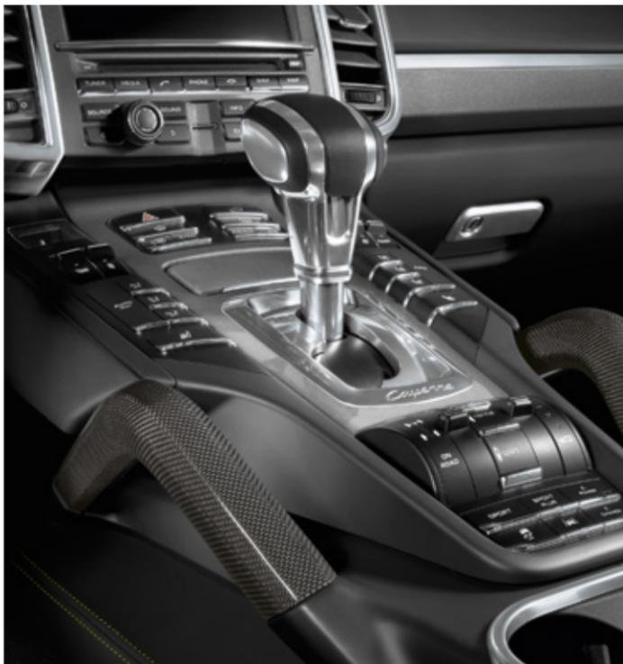
Extended interior package with grab-rails in carbon fiber and Tiptronic S gear selector in aluminum
