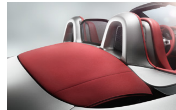
Roll-over bars painted in exterior colour, net-type wind deflector
