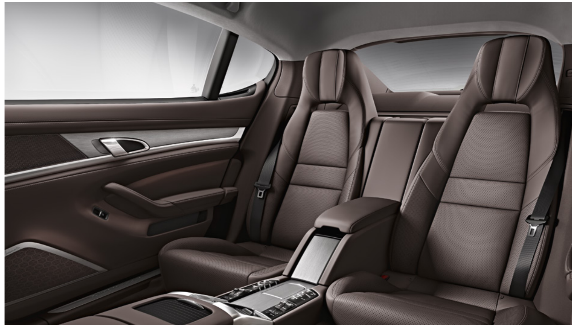
8-way power seats (rear) (in conjunction with large center console), with comfort headrests
