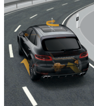
Porsche Torque Vectoring Plus (PTV Plus)
