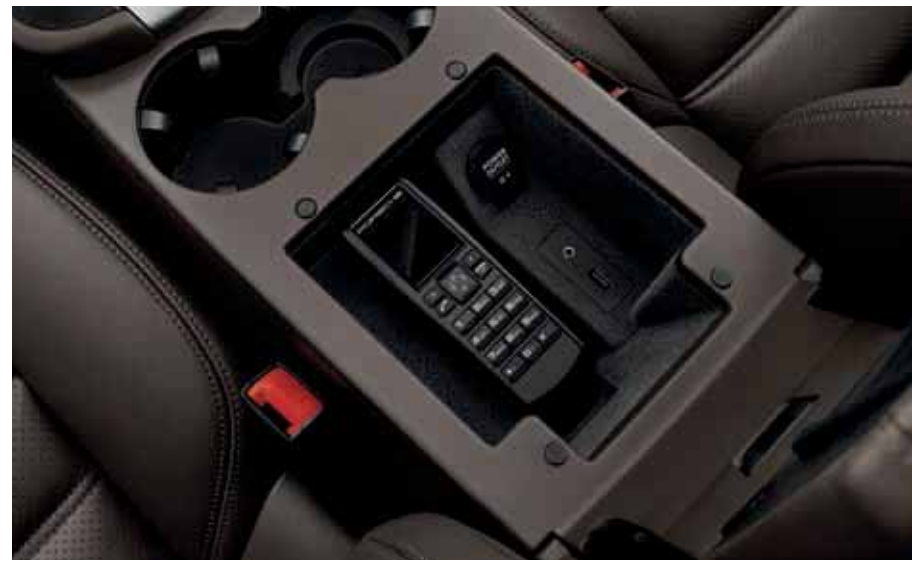
Telephone module with Bluetooth® handset
