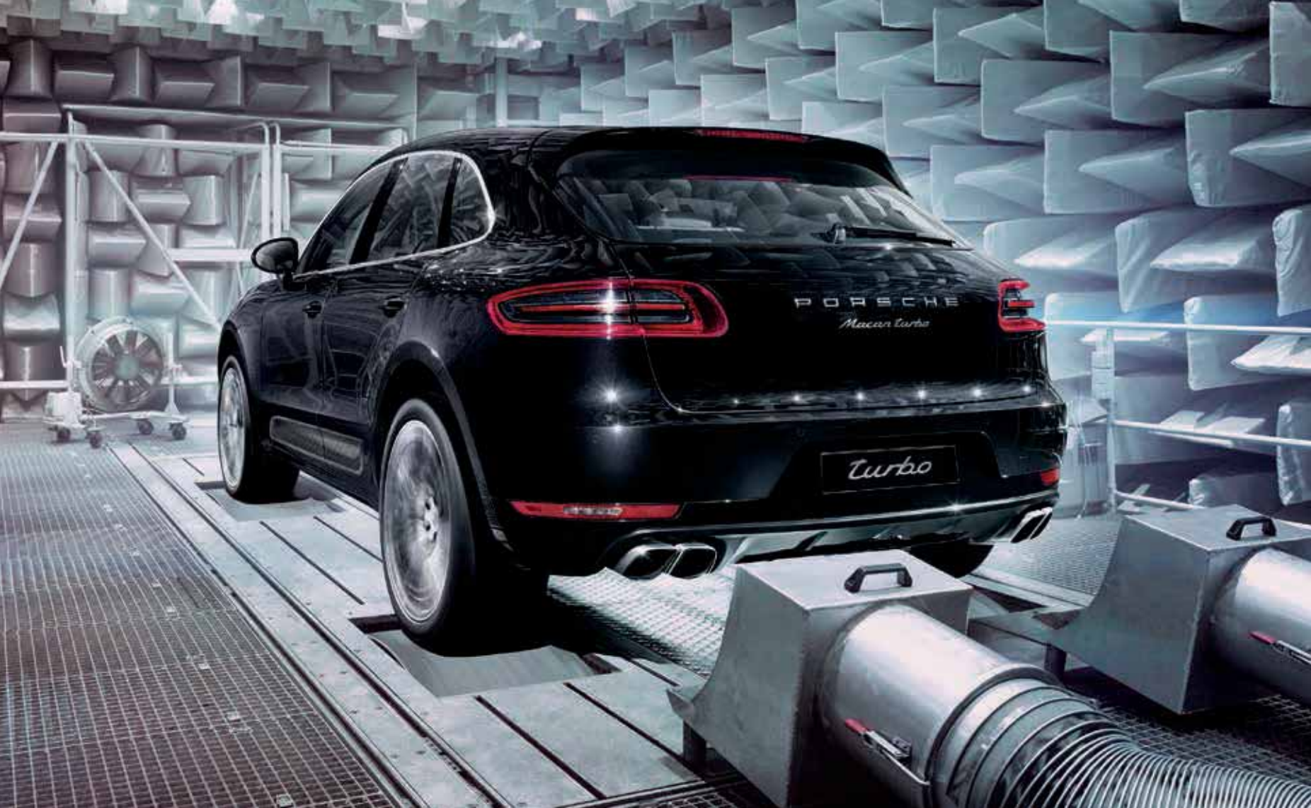
Acoustic test chamber in the Porsche Development Center, Weissach
