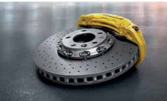
Porsche Ceramic Composite Brake (PCCB)
