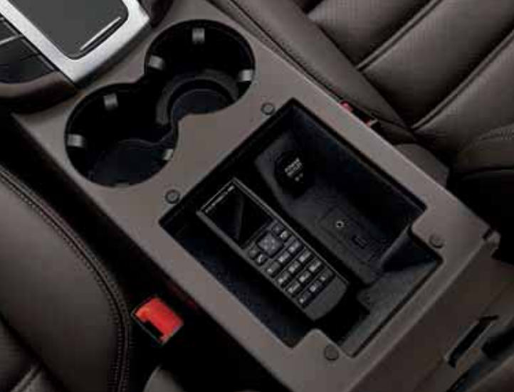
Telephone module (SAP and HFP) with Bluetooth® handset
