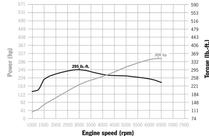
Cayenne: 295 lb.-ft. at 3000 rpm, 300 horsepower at 6300 rpm
