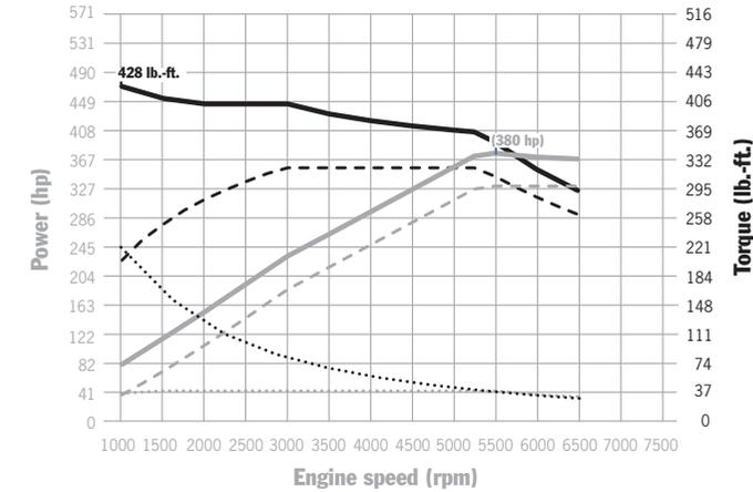
Cayenne S Hybrid: 428 lb.-ft. at 1000 rpm, 380 horsepower at 5500 rpm
