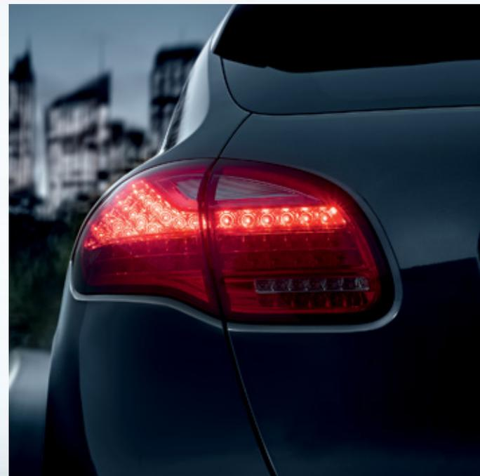
LED technology is used for all functions on the taillight modules. For an ultra-fast response and greater luminance.
