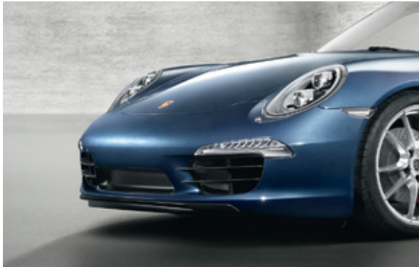
LED main headlights with Porsche Dynamic Light System Plus (PDLS+)
