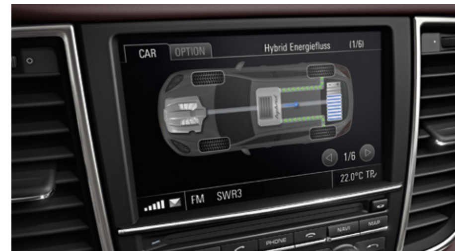
Display of the energy flow in the optional Porsche Communication Management (PCM)
