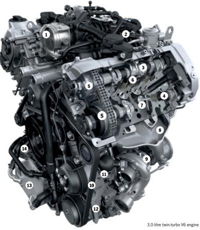
1. Throttle bodies/electronic throttle 2. Intake manifold 3. Intake camshaft 4. Exhaust camshaft 5. VarioCam Plus (valve adjuster) 6. VarioCam Plus (switching tappet) 7. Valve 8. Exhaust manifold 9. Turbocharger 10. Poly-V belts 11. PDCC/power steering pump 12. Air-conditioning compressor 13. Oil/water heat exchanger 14. Oil filter
