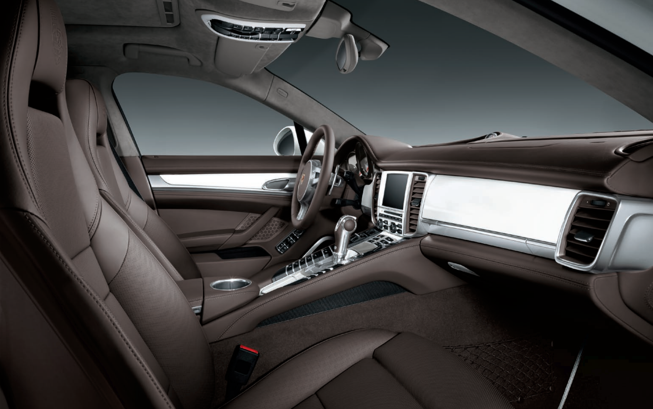
Interior package painted, PCM surround painted, dashboard trim package in leather, dashboard cover in leather, air vent slats in leather, steering wheel column casing and instrument cluster surround in leather, Porsche Crest embossed on front headrests, roofliner grab handles in leather, PDK gear selector in aluminium
