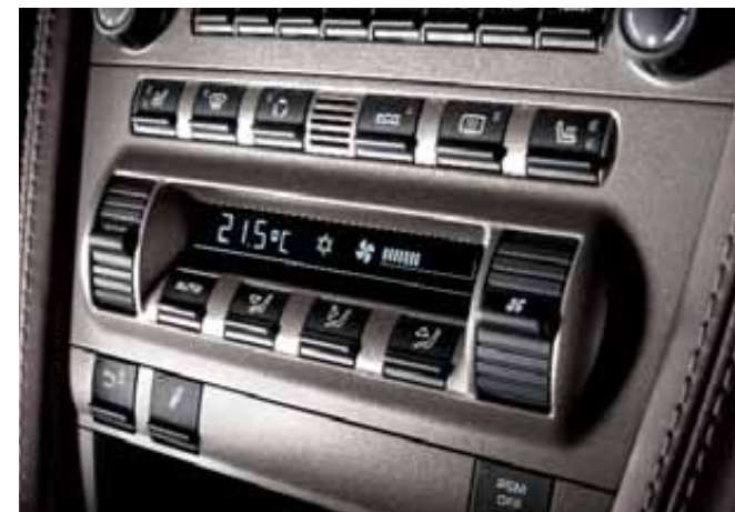
Automatic air conditioning
