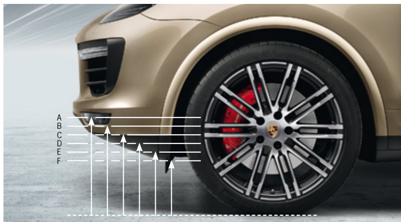
Air suspension with PASM. For greater driving dynamics and enhanced ride comfort (page 56). 1)
