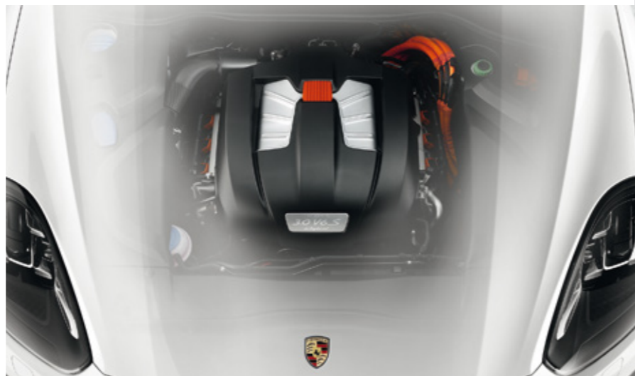
Cayenne S E-Hybrid (combined): 590 Nm between 1,250 and 4,000 rpm, 306 kW (416 hp) at 5,500 rpm
