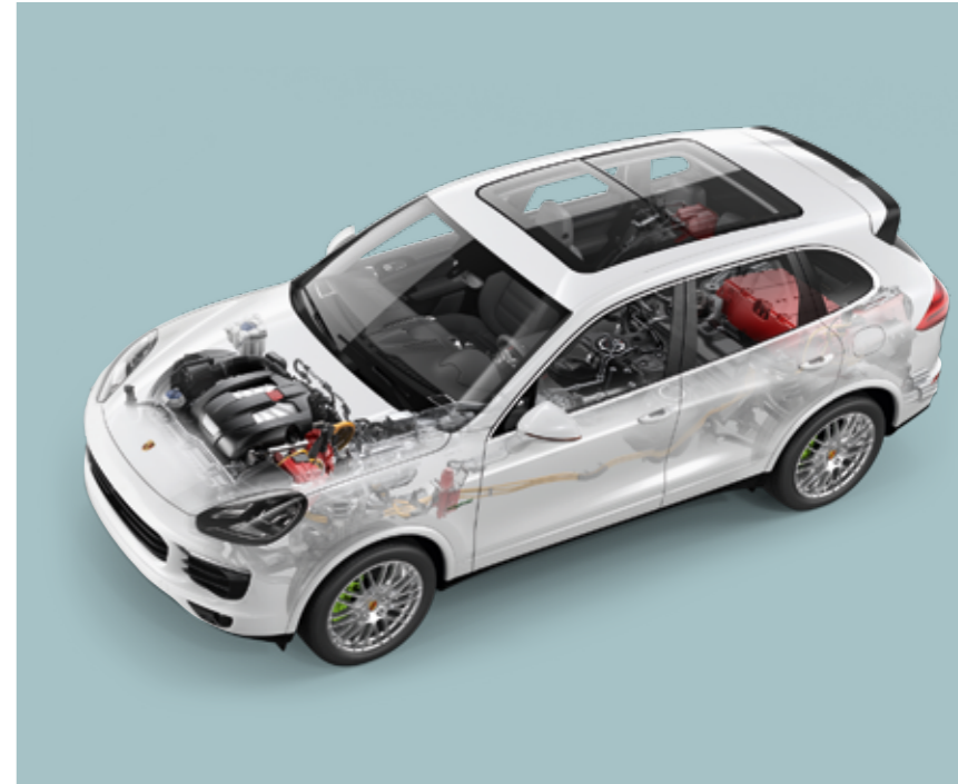
Drivetrain of the Cayenne S E-Hybrid
