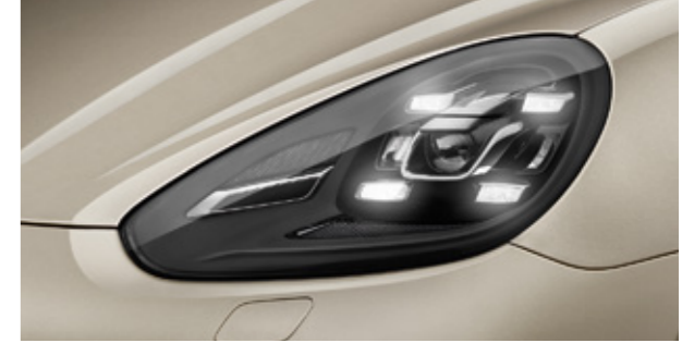
LED main headlights with Porsche Dynamic Light System Plus (PDLS+)
