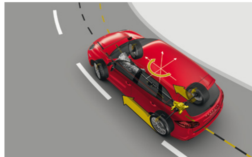
Porsche Torque Vectoring Plus (PTV Plus)
