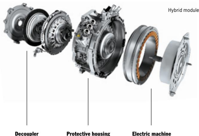
At 288 volts, the electric machine has a maximum output of 34 kW (47 hp). The benefits of the synchronous motor with inner rotor design are extremely compact dimensions and high levels of efficiency. It also acts as a starter motor and alternator.
