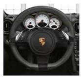
Three-spoke multifunction steering wheel for PDK
