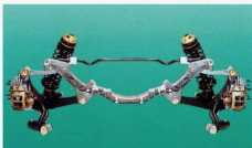
The ingenious Weissach rear suspension, designed in a competition among Porsche's R & D chassis engineers, increases stability while cornering - without the need for complex "active" electronics.
