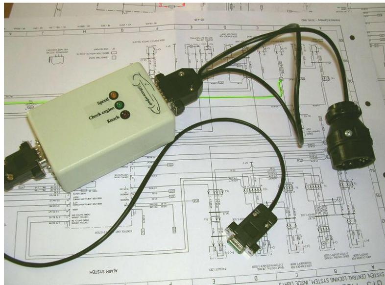
Interface module DT9xx with cables connected.
