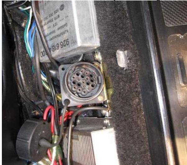
The 12 pin socket is located on the ecu mounting bracket very close to the EZK ecu.
