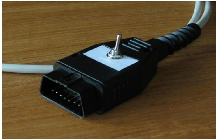
This is the 16P-OBDII connector with on top a switch to select one of the two diagnoses buses.
