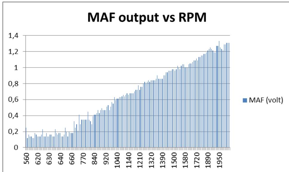
The engine will not cope with high rpm's so it is advised to only test this to about 2000 rpm.
