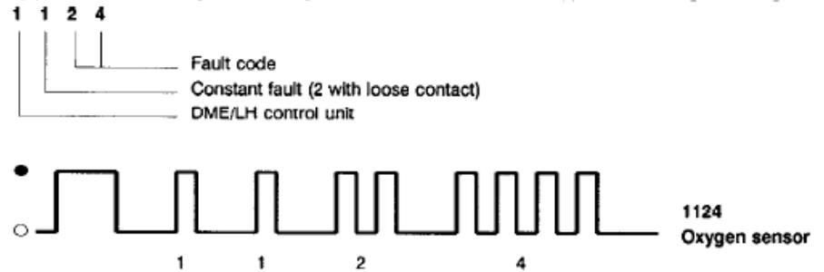
The check engine light can also be taken directly from the LH ecu pin 22. This is the signal linked to the MIL is presented in your 928 model. You can add a 12v LED to show it if required.
