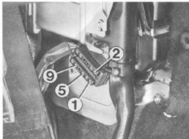
The optional 12pin rectangular cable has numbers on the socket assembly that provides orientation and proper installation. Please be aware that the connector must only be installed in the correct way. The pins in the connector must match the ones in the socket. It is as simple as that.
