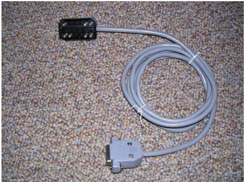
This is the 12pin diagnostic cable for the 1987/1988 928 models.
