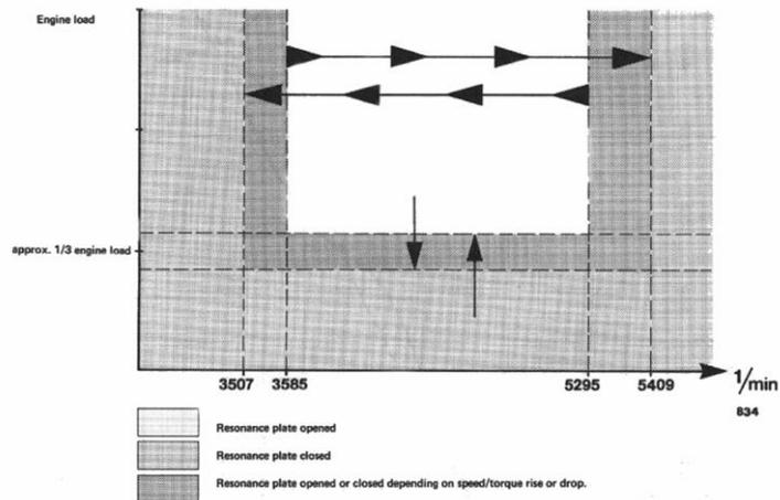
A system functional test is performed by clicking on the button “Resonance Flap”. This action can be heard as a rather loud click in the intake body, and seen when you remove the rubber cover on top of the intake manifold. It helps to make a marker on the axis of the flappy or attach a magnetic pointer. You will notice the axis of the flappy valve rotate 90 degrees. The test repeats itself every second until another function is selected.
