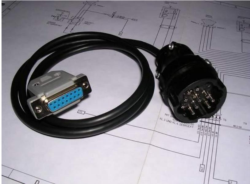
The interface cable DT9xx to the 19pin diagnostic socket
