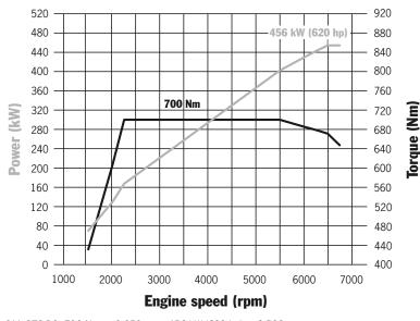
911 GT2 RS: 700 Nm at 2,250 rpm, 456 kW (620 hp) at 6,500 rpm
