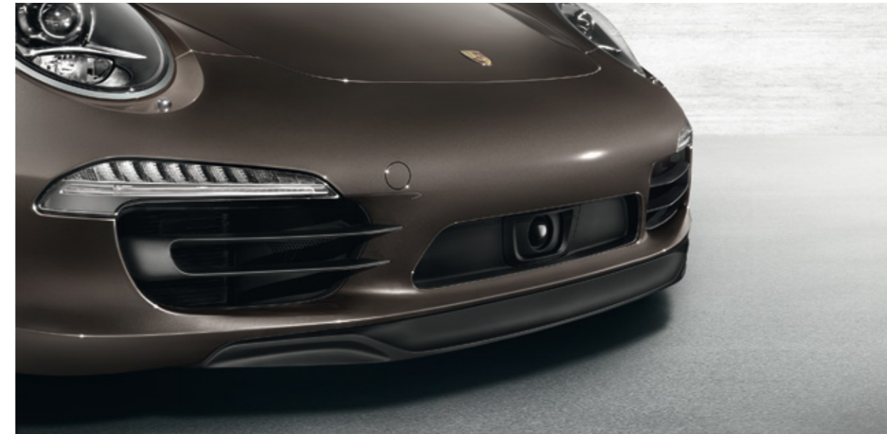
Radar sensor of adaptive cruise control
