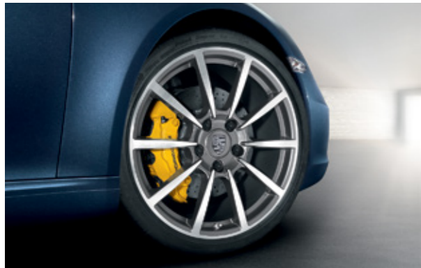
Porsche Ceramic Composite Brake (PCCB)
