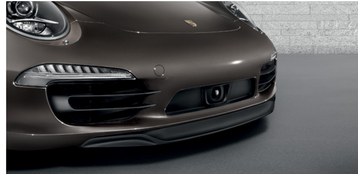
Radar sensor of adaptive cruise control
