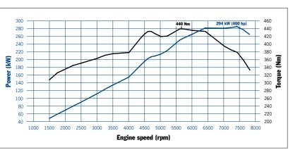
911 Carrera S: 440 Nm at 5,600 rpm, 294 kW (400 hp) at 7,400 rpm
