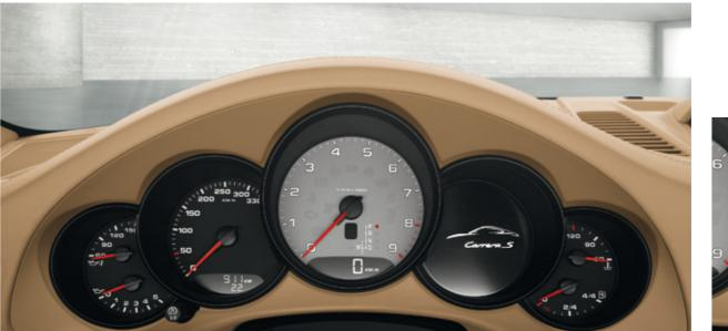
Instruments in the 911 Carrera S with aluminium-coloured rev counter
