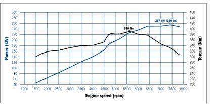
911 Carrera: 390 Nm at 5,600 rpm, 257 kW (350 hp) at 7,400 rpm
