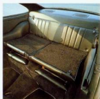
Rear seats can accommodate two adults for short journeys, or folded down, give increased luggage space.
