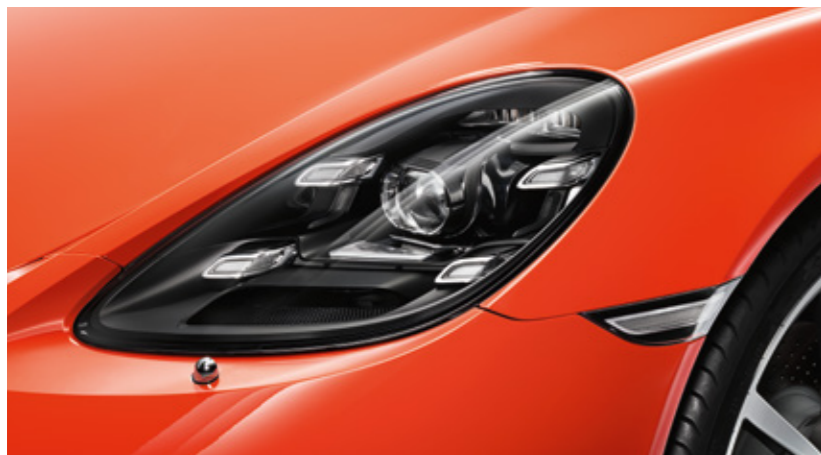
LED main headlights including Porsche Dynamic Light System Plus (PDLS Plus) (page 121)
