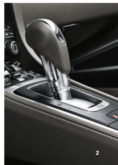
1 Gear lever for 6-speed manual transmission 2 Gear selector for Porsche Doppelkupplung (PDK)
